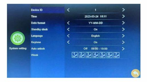
Door station parameter settings. Set the parameters of the door stations and the bell ringing tones.
